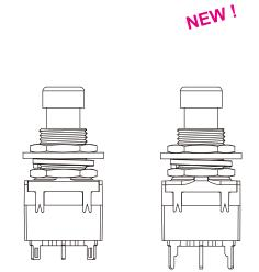
CONTACT RATING: 2A/4A 250/125VAC, 2A/4A 24/12VDC. ELECTRICAL LIFE: 20,000 make-and-break cycles at full load. CONTACT RESISTANCE: 50m-ohms max. initial @2-4VDC INSULATION RESISTANCE: 500VDC 100M-ohms min. DIELECTRIC STRENGTH: 1,500VAC for 1 minute.
