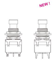
CONTACT RATING: 2A/4A 250/125VAC, 2A/4A 24/12VDC. ELECTRICAL LIFE: 20,000 make-and-break cycles at full load. CONTACT RESISTANCE: 50m-ohms max. initial @2-4VDC INSULATION RESISTANCE: 500VDC 100M-ohms min.
